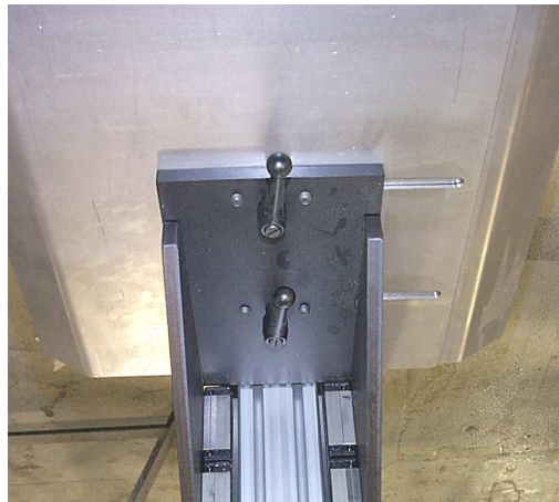
Figure 3.1 – Lower mouth adjusting handles
