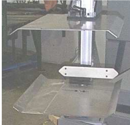
Figure 3.0 – Upper and lower stainless steel mouth.
