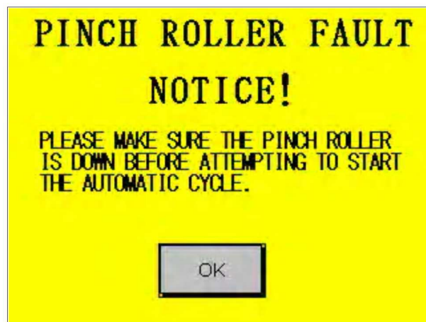
Figure 3.6: Pinch Roller Fault
