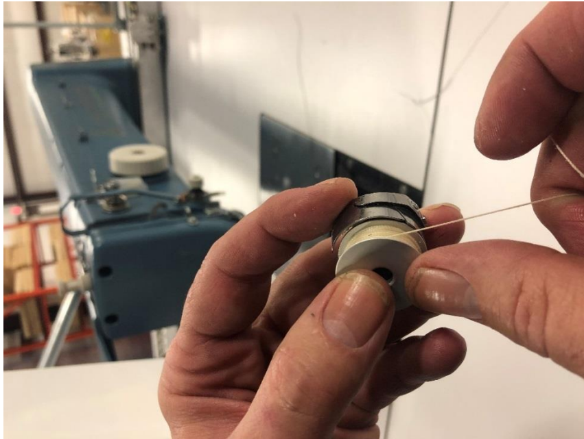
(ref. 3.5) Take out the old bobbin and replace it with a new bobbin so that it rotates clockwise.
