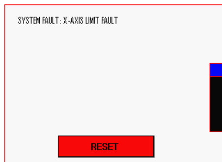
Figure 3.21: Major fault screen
